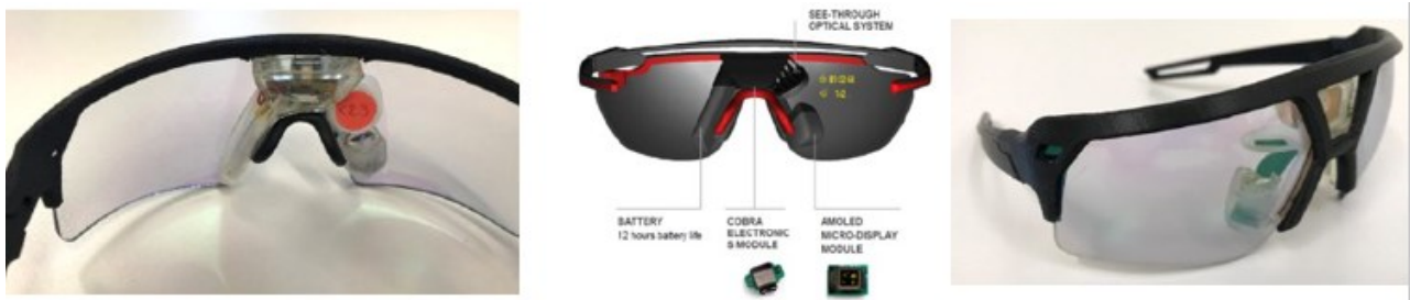
Figure 2: AR glasses with a monochromatic field of view
